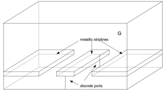
**Fig. 1.** Coplanar waveguide.
