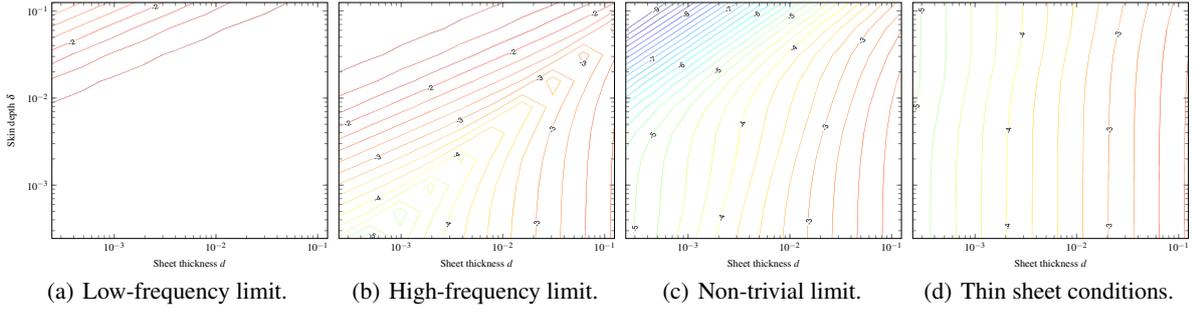
**Fig. 2.** The modelling error when using (a) the low-frequency limit, (b) the high-frequency limit, (c) the non-trivial limit, and (d) the thin sheet conditions (3) to approximate the shielding of conducting sheets of different thicknesses  $d$  and different frequencies or skin depth  $\delta$ . The shown error is the one of the magnetic field outside the thin sheet.
