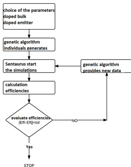
Fig. 2. flow chart simulator device and genetic algorithm
