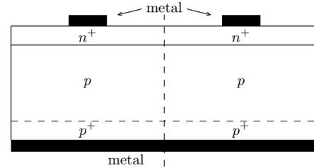
**Fig. 1.** Geometry of the test photovoltaic cell
